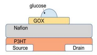
Figure 15: The OTFT Structure
