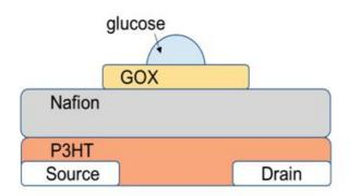
Figure 15: The OTFT Structure
